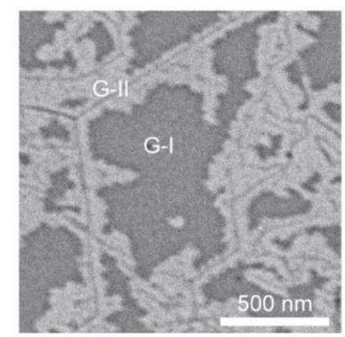
Two distinct graphene regions: G-I on the sapphire terraces G-II close to the sapphire step edges
