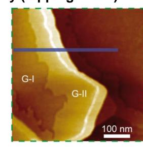
Large-area AFM images (left) show homogeneous SLG without signs of cracks or defects confirming the Raman results. Sapphire step edges and capillary wrinkles can be observed. In the higher resolution AFM image (middle) a vertical height variation between two graphene regions is visible.
